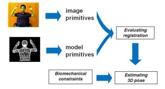
Fig. 2. The implemented approach for 3D motion capture
